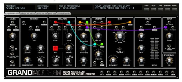
To draw a patch cable, click on an output patch point, keep the mouse button pressed, drag the cable to a patch input point then release the mouse button.
